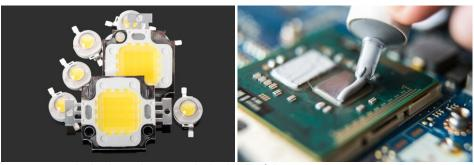
Fig 2.1.10: Apply the thermal paste on the back side of the COB
