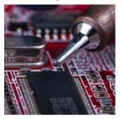
Fig1.3.4: Solder Iron Tip
