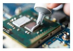
Fig 2.1.4: Thermal Grease.
